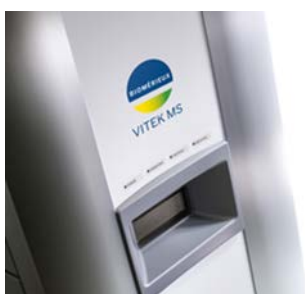
Figure 2. Biomerieux Vitek MS – an automated mass spectrometer.
